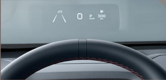
The Head-Up Display (HUD) projects key driving data onto the windshield, keeping essential information in view for safer, more focused, and convenient driving.
